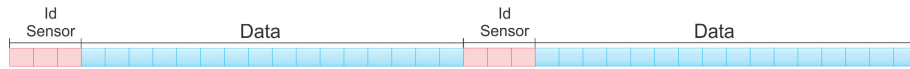
FIGURE 13. Frame structure for sending regular sensor information. Organization of the data field for sending values from: two regular sensors.
