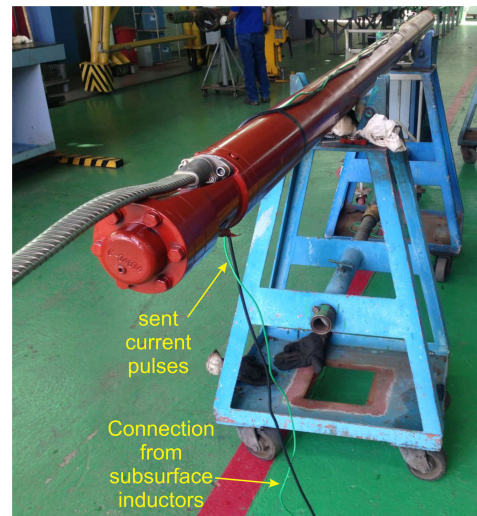
FIGURE 5. ESP components: Motor-pump assembly installed horizontally.
