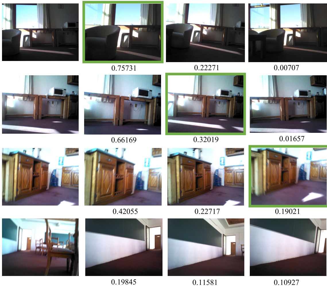
FIGURE 7. Localization results using the CIMAT-NAO-A dataset. At left: Query image, next three images: Top-3 class probabilities. Under each retrieved key-image, the probability is shown. In a green box, the ground-truth key image is highlighted. The last row indicates when the top-3 retrieved key images are not the ground-truth localization key image.
