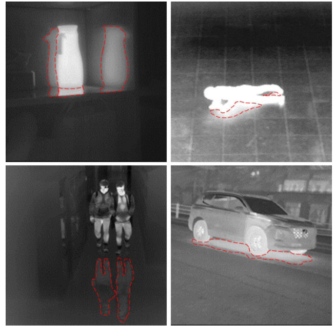
FIGURE 1. Examples of 1-channel thermal images with thermal reflections (red dashes) and objects.
