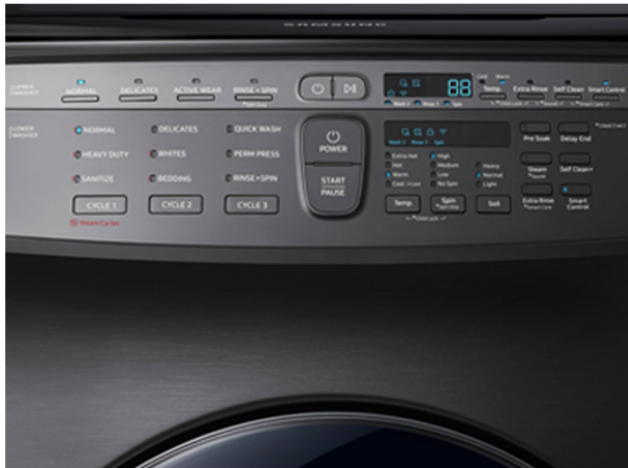
FIGURE 1. An example washing machine user interface for selecting preferred mode of operation. The user has to manually select multiple options before the washing is enabled. Our auto-completion solution will reduce the number of manual operations on the WM.
