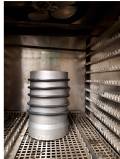
FIGURE 2. Cable samples inside the oven for combined aging.
