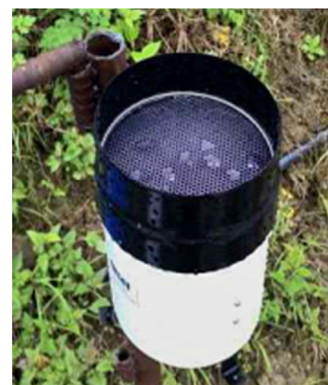
FIGURE 7. The on-site rainfall automatic rain gauge layout diagram.
