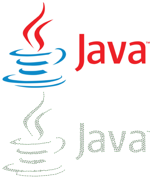
FIGURE 10. Topological feature extraction of input image based on the SA-GNG algorithm. The topology network of 543 nodes is generated automatically, and the information entropy H(X) is 0.998.
