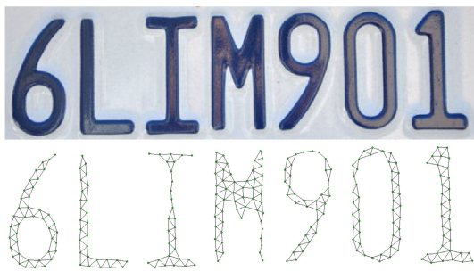
FIGURE 7. Topological network of 264 nodes is automatically generated to extract the digital features of the license plate, and the information entropy H(X) is 0.998.
