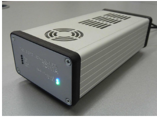
FIGURE 14. Arduino-Due based thermo-opto-mechanical laboratory system TOM1A.
