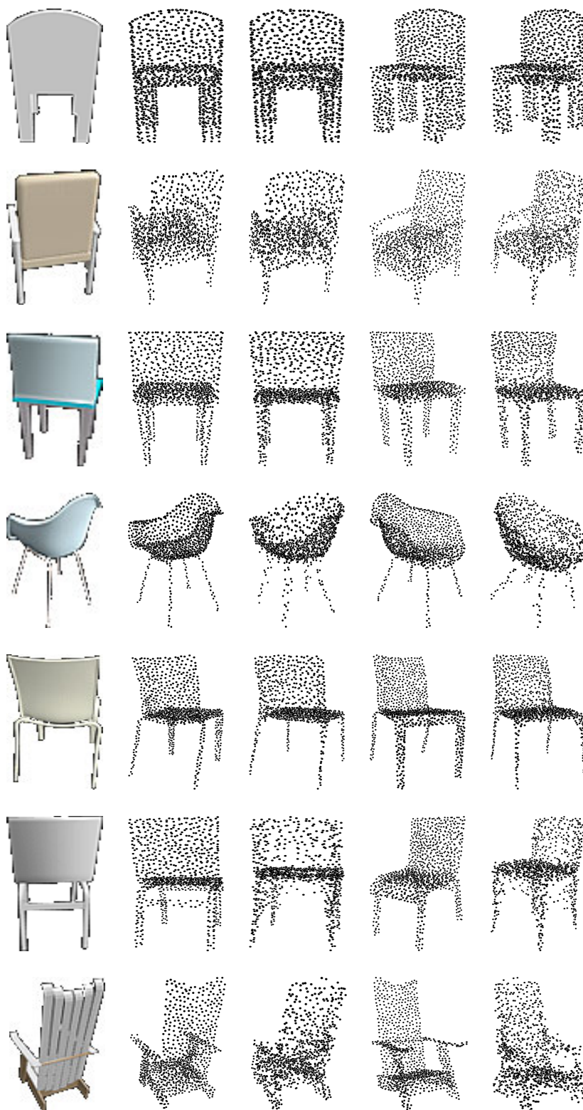
FIGURE 6. Qualitative results of 3D reconstruction for the ambiguous 2D inputs. From left to right: 2D input image, ground-truth view-1, generated output view-1, ground-truth view-2, generated output view-2.
