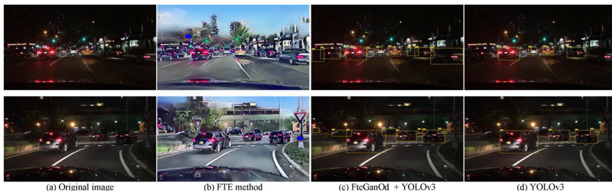
FIGURE 8. Detection results from DATASET1 (hard): (a) Original image. (b) FTE results. (c) Detection results with FteGanOd + YOLOv3. (d) Detection results with YOLOv3.
