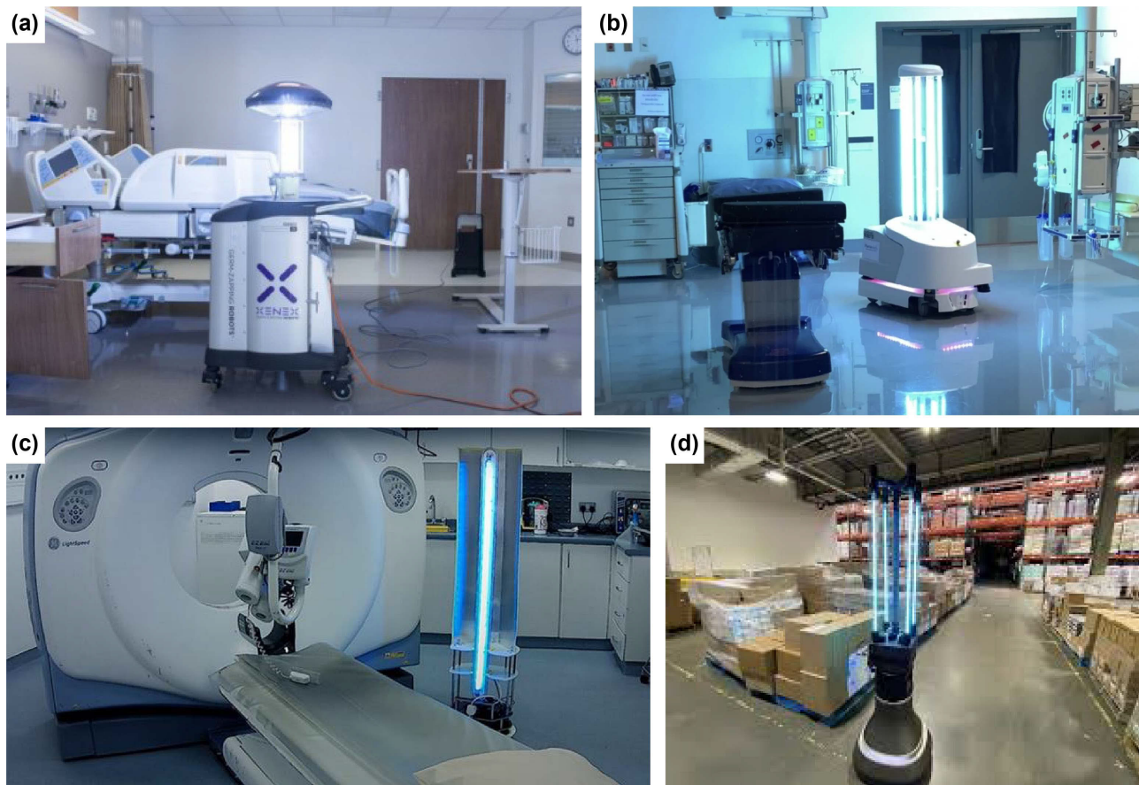
FIGURE 4. UV-C robots. (a) Xenex light strike robot (photo credit: Xenex). (b) UVD robot moving and disinfecting a surgery room (photo credit: UVD Robot). (c) Akara robot disinfecting corners in a laboratory room (photo credit: Akara Robotics). (d) MIT UV robot disinfecting food bank (photo credit: MIT).
