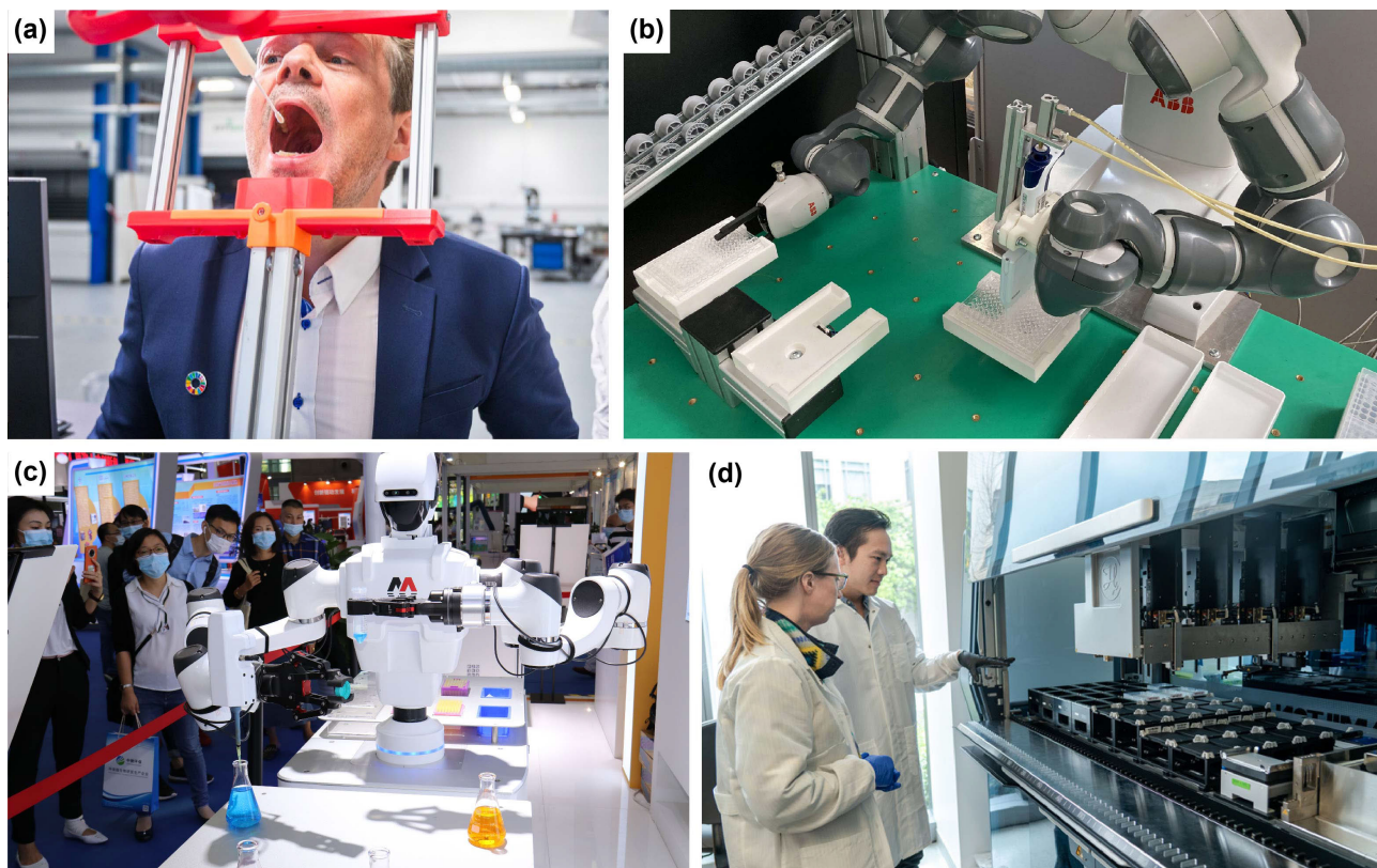
FIGURE 2. Robots for COVID-19 diagnosis. (a) Lifeline Robotics' throat swabbing robot collecting a sample (photo credit: The Maersk Mc-Kinney Moller Institute at the University of Southern Denmark) [44]. (b) ABB's collaborative robot, YuMi [55], was used in an application designed at the Politecnico di Milano, in partnership with IEO to support hospitals in serological testing (photo credit: Cristina Perini) [42]. (c) MOD Robot by Moying Robotics, Shenzhen, China (photo credit: Dr. Yiming Yang). (d) An automated liquid-handling robot (Hamilton STARlet) that will be used to analyze swabs from patients to diagnose COVID-19 (photo credit: Max & Jules Photography) [56].
