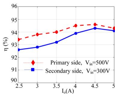
FIGURE 23. Efficiency results of the proposed converter.
