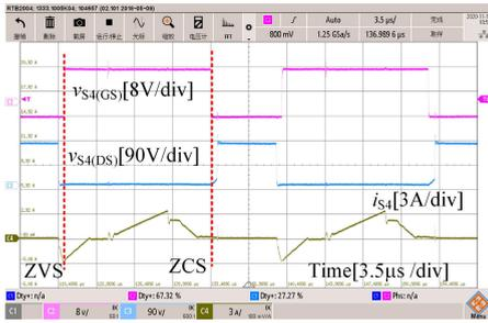
FIGURE 20. ZVCS of  $S_4$  in the primary side modulation mode.
