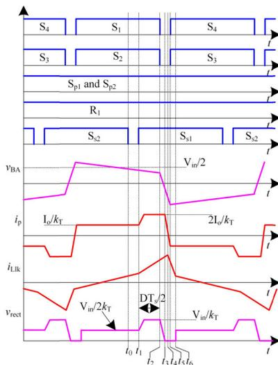
FIGURE 3. Core waveforms in the secondary side modulation.
