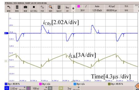
FIGURE 19.  $i_{Cfly}$  and  $i_{Llk}$  in the primary side modulation mode.
