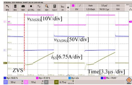
FIGURE 14. ZVS of  $S_3$  in the secondary side modulation mode.
