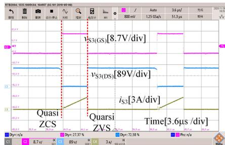
FIGURE 21. ZVCS of  $S_3$  in the primary side modulation mode.
