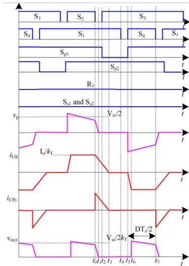
FIGURE 2. Core waveforms in the primary side modulation.
