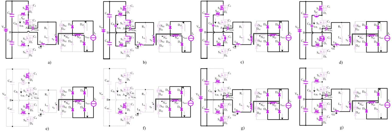
FIGURE 4. Power stages in the primary side modulation: a) stage 1; b) stage 2; c) stage 3; d) stage 4; e) stage 5; f) stage 6; g) stage 7; h) stage 8.
