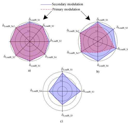
FIGURE 11. Soft-switching load range of the primary switches: a) proposed; b) Fig.6 (a); c) Fig.6 (b).
