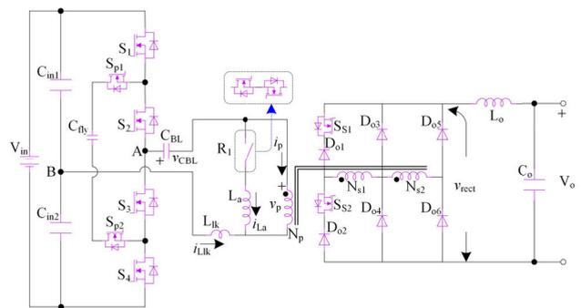
FIGURE 1. Flexible structure TL dc-dc converter.
