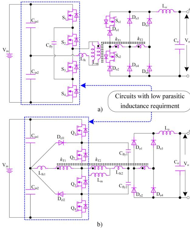
FIGURE 6. Circuit for comparison: 1) converter in [12]; 2) converter in [28].
