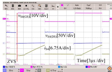
FIGURE 15. ZVS of  $S_4$  in the secondary side modulation mode.
