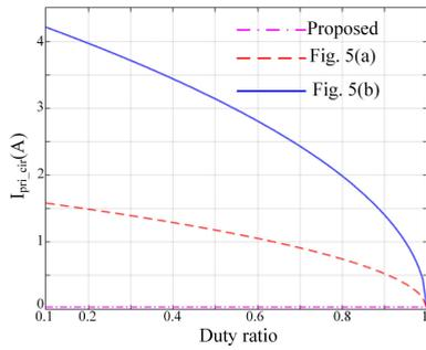
FIGURE 10. Primary circulating current vs. duty ratio.
