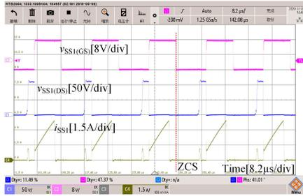
FIGURE 16. ZCS of  $S_1$  in the secondary side modulation mode.
