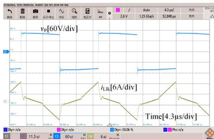
FIGURE 12.  $v_p$  and  $i_{Llk}$  in the secondary side modulation mode.
