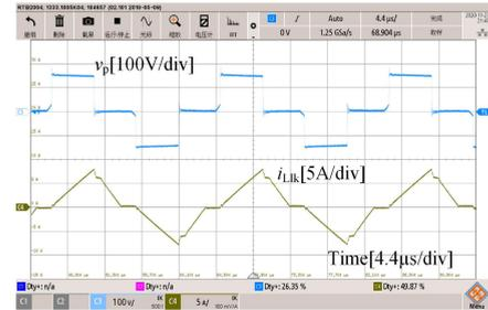
FIGURE 18.  $v_p$  and  $i_{Llk}$  in the primary side modulation mode.
