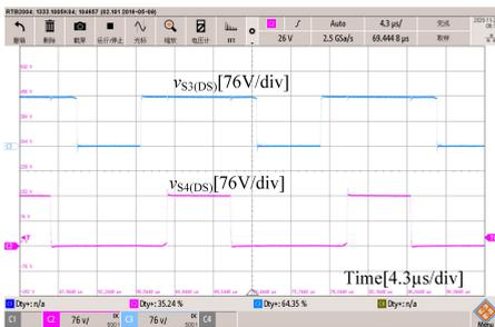
FIGURE 22.  $v_{S4(DS)}$  and  $v_{S3(DS)}$  in the primary side modulation mode.
