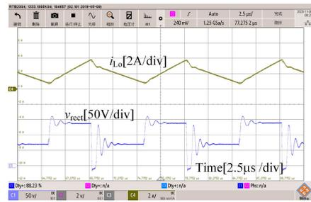
FIGURE 13.  $V_{rect}$  and  $i_{Lo}$  in the secondary side modulation mode.
