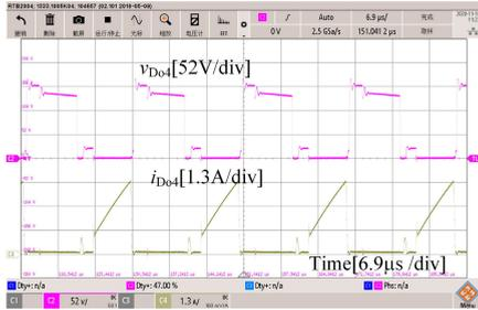
FIGURE 17.  $v_{D04}$  and  $i_{D04}$  in the secondary side modulation mode.
