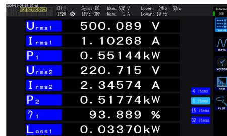
FIGURE 25. Hard copy of the efficiency result.
