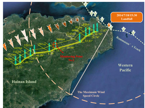
FIGURE 14. The 110kV double-circuit transmission line.
