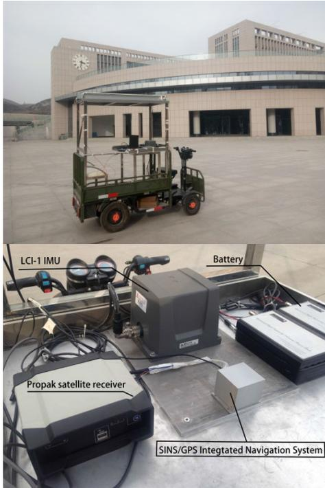
FIGURE 5. The car-mounted experimental platform.
