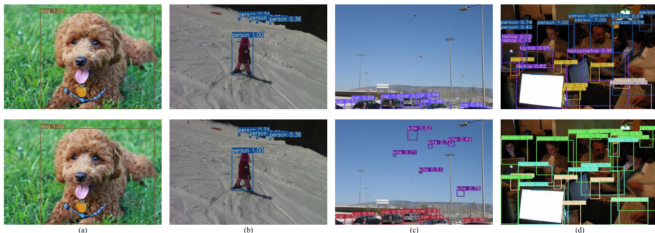
FIGURE 9. Comparison of the detection results of YOLOv3 (the top row) and YOLO-ACN (the bottom row) on typical images on the test set of MS COCO 2017. The detection result of the large size object in the (a) are similar, and the small objects can also be detected well with the proposed YOLO-ACN network, e.g., the long-distance person in (b); the kites and cars in (c); the cups and laptops in (d).
