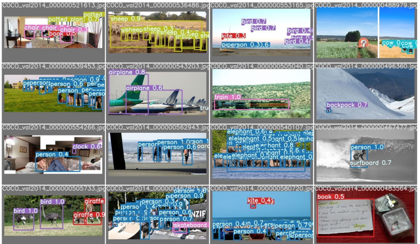
FIGURE 8. YOLO-ACN test results on the validation set of MS COCO 2014. When the first batch training is completed, these images are randomly selected for testing. From the test results, although only one batch is completed, most objects can be detected, especially small targets and occluded objects.
