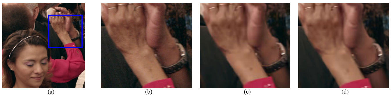
FIGURE 12. Subjective visual comparisons with some decoded frames at QP = 37 under AI. (a) Original 72-th frame of Tango2 (3840 × 2160) (cropped), (b) Original frame (enlarged), (c) Ours (enlarged decoded frame; 38.36 dB), and (d) the default RC method (enlarged decoded frame; 38.28 dB).
