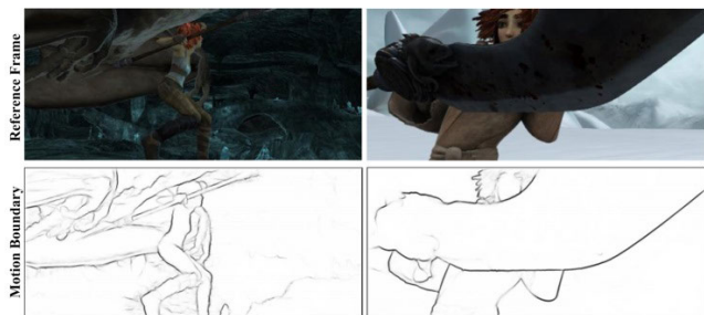
FIGURE 5. Estimated motion boundary of the MPI-Sintel datasets. Top is the reference frame and bottom is the estimated motion boundary. FIGURE 6. Flow fields of the various ablation models on some MPI-Sintel training sets. From top to bottom: sequences of alley_2, cave_4 and market_6.
