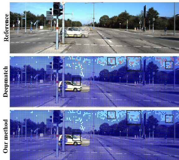
FIGURE 4. Illustration of the proposed grid-based neighboring support optimization in improving the accuracy of matching field, where the blue mark indicates the correct matching pixel and the red mark denotes the incorrect matching pixel.
