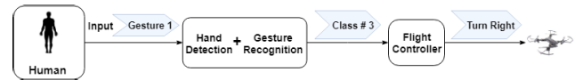
FIGURE 7. The experimented case: penalty on the classifier. The commands are: class #0: Take-off, class #1: Land, class #2: Turn left, and class #3: Turn right.
