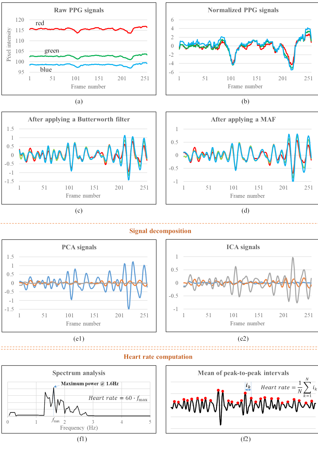
FIGURE 3. Process flows of the PPG methods (M4 and M5) in Table 1. M4 is represented by processes from (a) to (e1) and (f1). M5 is represented by processes from (a) to (e2) and (f2).
