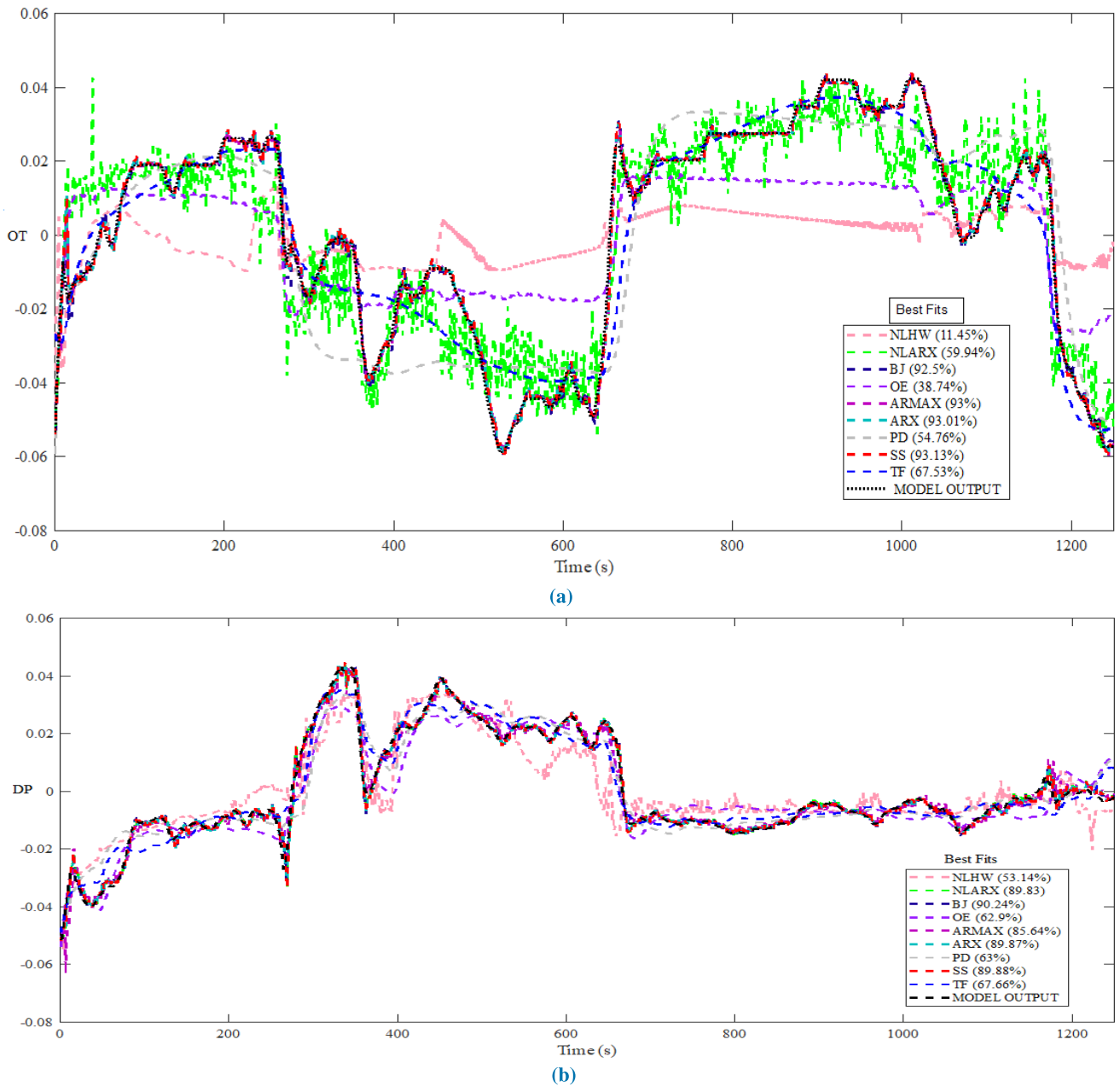
FIGURE 7. The model fit percentage using different system identification methods (a) for OT (b) for DP.
