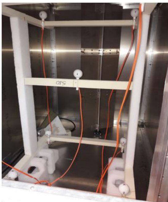
FIGURE 7. Multi-probe setup in a classical RC [25].
