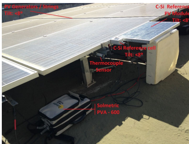
FIGURE 4. The c-Si solar PV cell and PV module (coplanar to the PV generator), thermocouple sensor, and Solmetric (PVA 600) commercial capacitive load.
