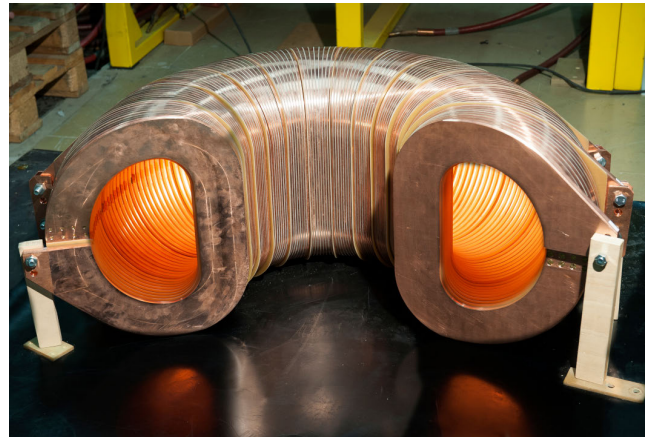
FIGURE 5. Unfinished toroidal inductive storage (12 of 20 modules).
