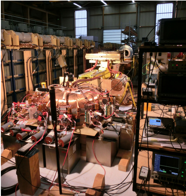
FIGURE 8. XRAM generator connected to the railgun RAFIRA.
