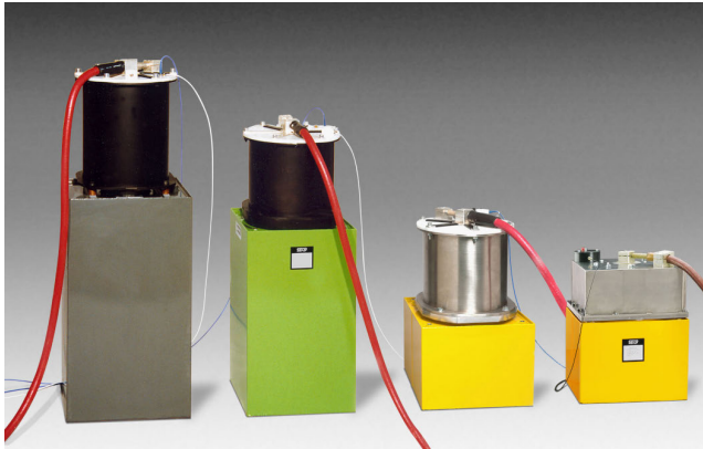
FIGURE 3. Development steps of 50 kJ capacitive PFUs at ISL [48].
