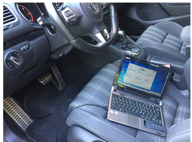
FIGURE 7. The setup connection between the car, OBD-II interface and VCDS GUI.
