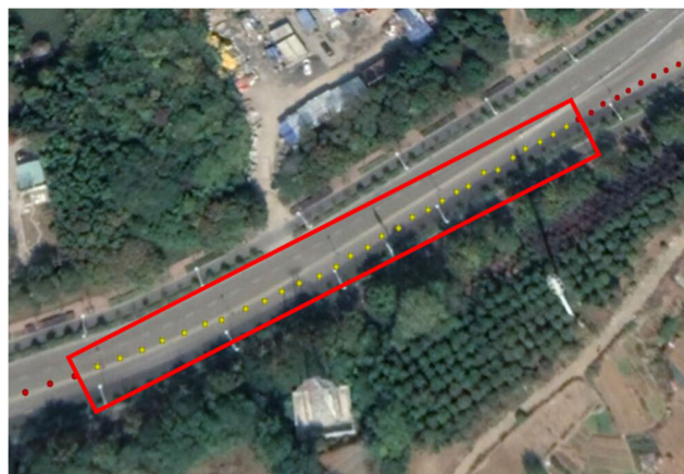
FIGURE 2. Positioning processed with inter-system differencing algorithm. The yellow dots in box can't obtain results with classical loose combination model.
