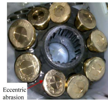
FIGURE 2. Slipper's eccentric abrasion and failure picture.
