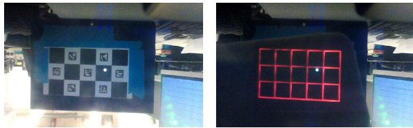
(a) Captured real ChArUco board (b) Captured virtual grid with see-through virtual contents hidden
