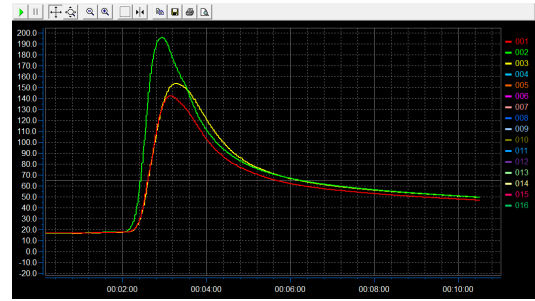
FIGURE 20. Three-phase winding temperature rise for SPM machine when the torque is 35Nm.
