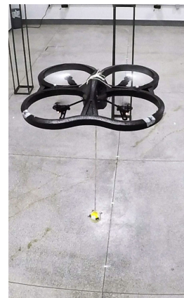
FIGURE 5. Photo of the quadrotor and the load used in the experiments.
