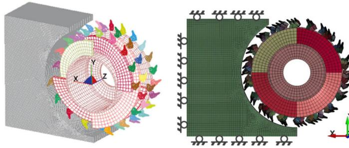
FIGURE 2. FEM model and boundary conditions of the drum cutting coal.
