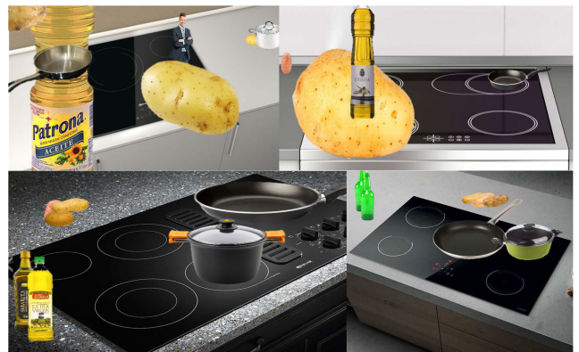
FIGURE 6. Example of some of the occlusions found in the automatic synthetic dataset (top) and realistic synthetic dataset (bottom). Top: Since the objects are randomly distributed, these occlusions are also random. The maximum allowed level of occlusion can be modified with a parameter. Bottom: These occlusions appear similar to those we can find in reality.
