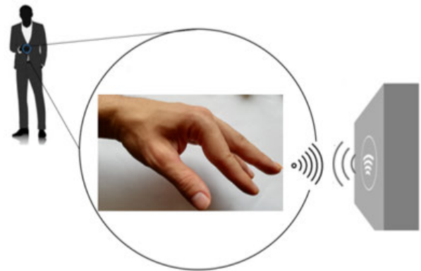
FIGURE 1. Illustrative on-fingernail antenna communication environment.
