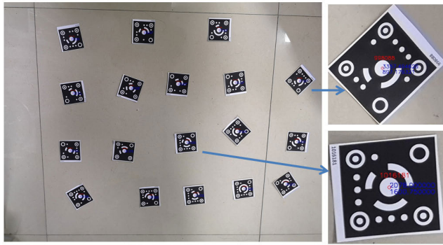
FIGURE 9. The recognition result with the ground as the background, the centers of the coded targets are targeted using red circles and the center coordinates and the codes are written on the image using blue and red respectively.
