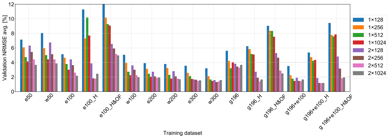
FIGURE 10. Average validation NRMSE of models with different sizes and trained on datasets constructed with different methods and number of samples.
