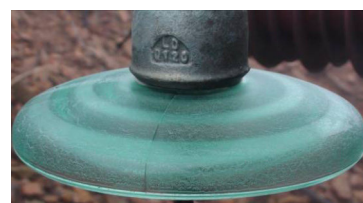
FIGURE 2. Surface of an insulator wetted by natural fog.
