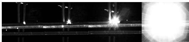
FIGURE 13. Consecutive record of arc evolution (interval was 20ms).
