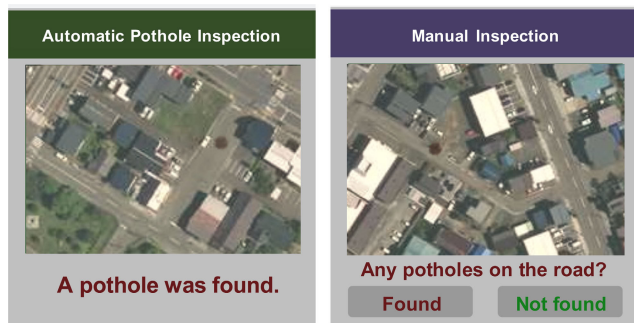
FIGURE 6. Pothole inspection. Automatic inspection result window (left). Manual inspection window (right).
