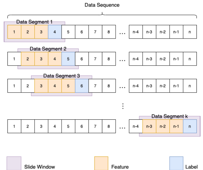
FIGURE 3. Sliding window method to generate data segments.
