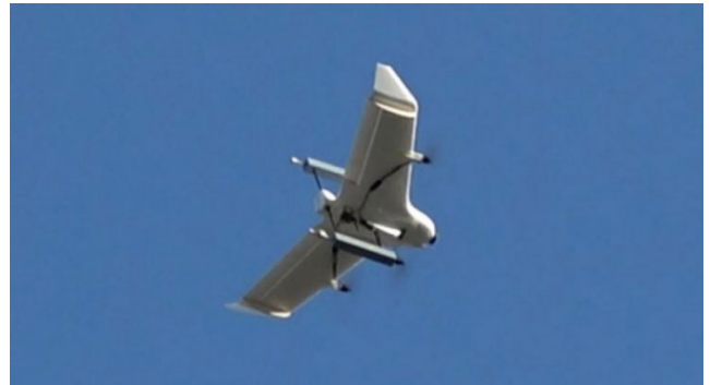
FIGURE 1. The tail-sitter UAV in cruise.
