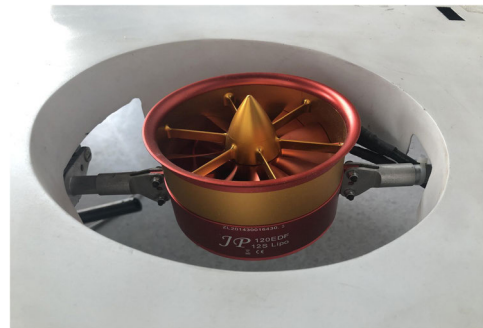
FIGURE 7. The configuration of rear ducted fan.
