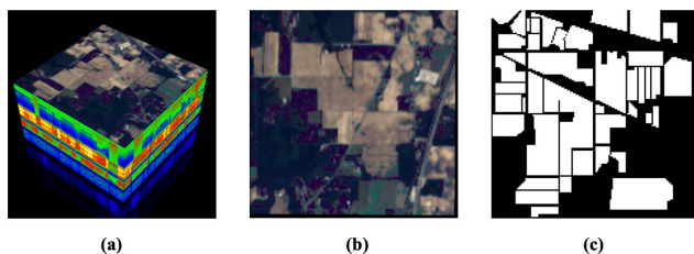
FIGURE 10. The sample of hyperspectral image (Indian Pine Site 3 AVIRIS hyperspectral dataset). (a) overview image, (b) cross section, (c) ground truth.
