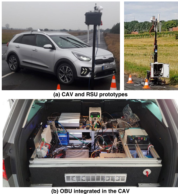
FIGURE 5. Prototypes used to collect V2X messages.
