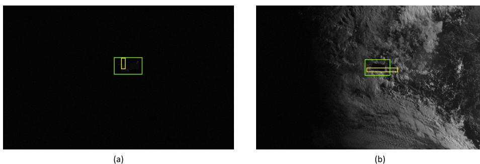
FIGURE 18. Failed cases in spacecraft detection: (a) Poor light condition and small object; (b) Earth background and small object. (Green bounding box denotes ground truth; yellow bounding box denotes wrong box.)
