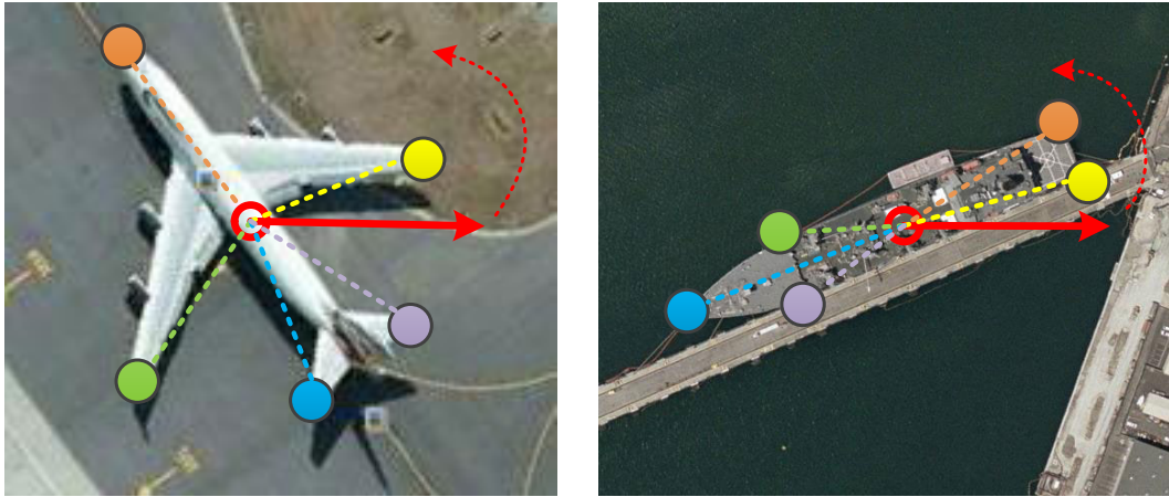
FIGURE 9. In polar coordinates, P-RSDet can be transplanted to more precise keypoint detection tasks by simply increasing the number of polar radius \rho and polar angles \theta in regression.
