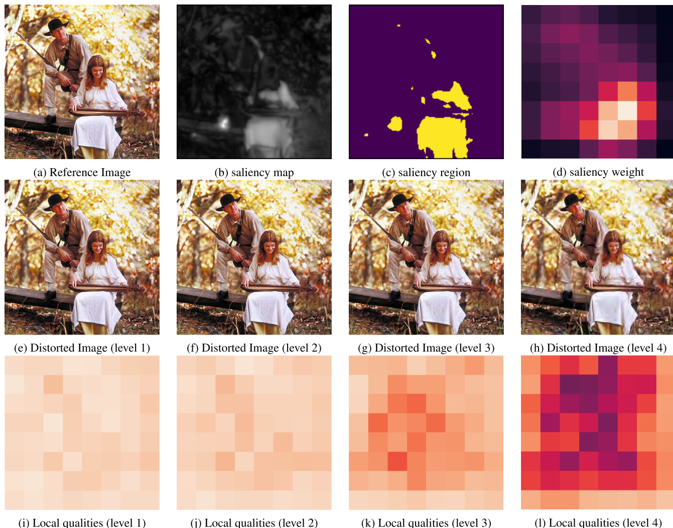
FIGURE 13. Local qualities and saliency weights for a JP2K distorted image from CSIQ. The clors black and white indicate low and high values of local qualities respectively. The DMOS values are 0.9978, 0.9274, 0.6141, 0.3693 in range [0;1], predicted qualities are 47.7512, 46.7519, 42.5574, 32.1268 in range [10;50].
