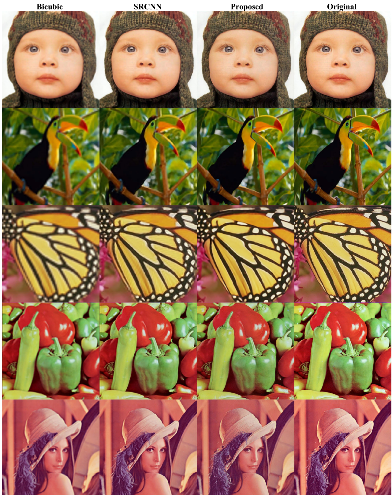
FIGURE 7. Partial super-resolution reconstruction results of the Set5 and Set14 datasets. From left to right, the images correspond to those obtained using the bicubic model, SRCNN model, and proposed model, and the original HR image. The proposed method yields sharp results with higher quality and richer texture details, while the images obtained using the other models are blurry.
