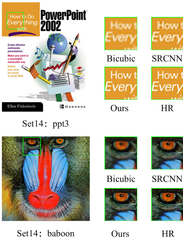
FIGURE 4. Comparison of the magnified reconstruction results of different SR methods: Super-resolution results of 'ppt3' (Set14) and 'baboon' (Set14) with a scale factor of \times 4 . Top: The texts obtained using the proposed method are sharp; the character edges corresponding to the other methods are blurry. Bottom: The proposed method recovers sharp results, while the other models yield blurry results.
