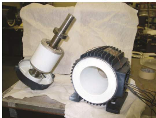
FIGURE 11. Encapsulated rotor and stator as previously studied by [66] (©2011 IEEE).
