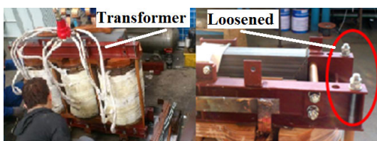
FIGURE 20. Transformer disassembly inspection experiment.
