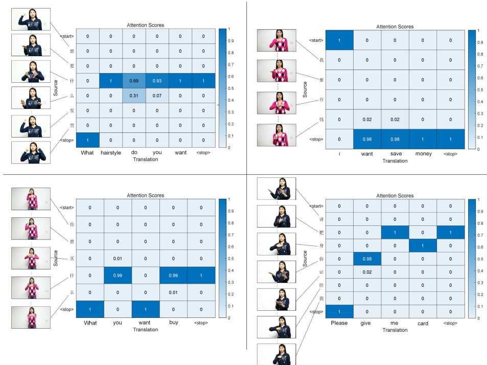
FIGURE 8. Example attention score matrix. The proposed end-to-end sign language translation system can translate key words well by using the attention mechanism.
