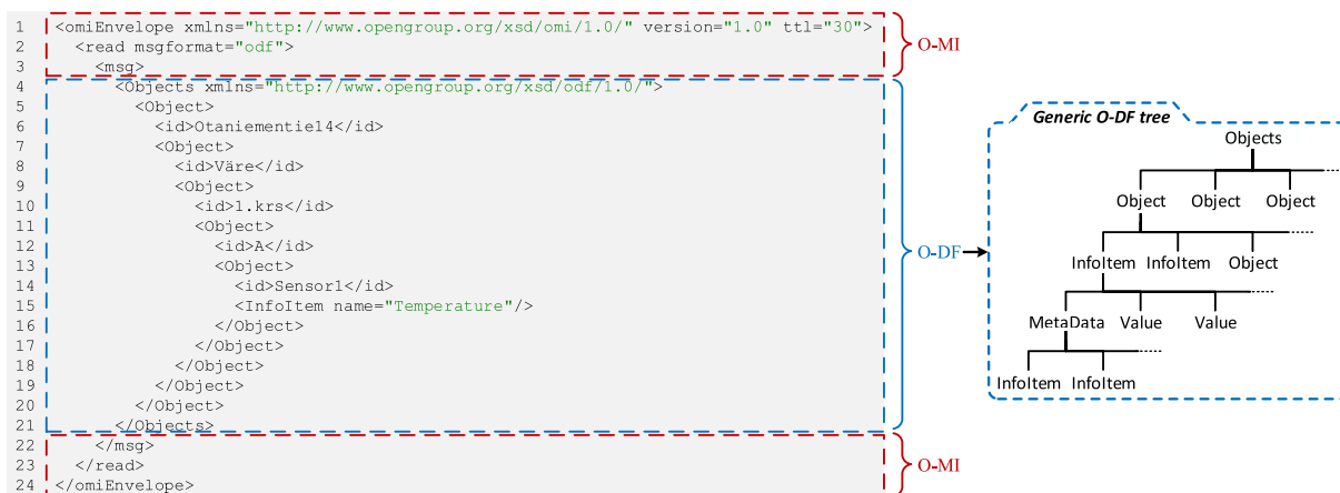
FIGURE 4. O-MI/O-DF read message requesting for temperature data.
